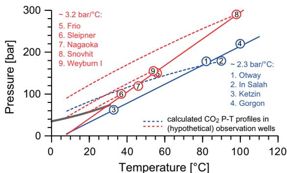
**Fig. 8.** Compilation of initial reservoir P–T conditions of different CO<sub>2</sub> storage sites and calculated exemplary CO<sub>2</sub> P–T paths in hypothetical observation wells (see text for details). The initial reservoir P–T conditions define two different initial pressure–temperature gradients of ~2.3 and 3.2 bar/°C, respectively.
