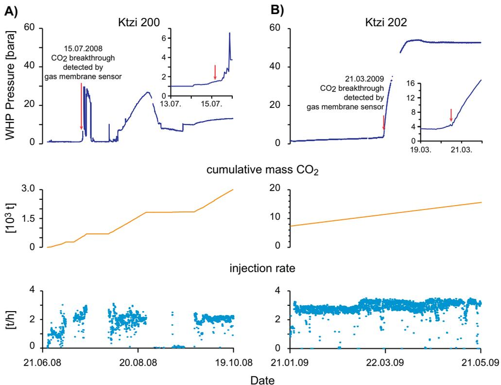
**Fig. 6.** Wellhead pressure recordings during arrival of CO<sub>2</sub> in observation wells (A) Ktzi 200 and (B) Ktzi 202. Arrival of CO<sub>2</sub> in both observation wells has been detected with a gas membrane sensor installed at 150 m depth in the wells.
